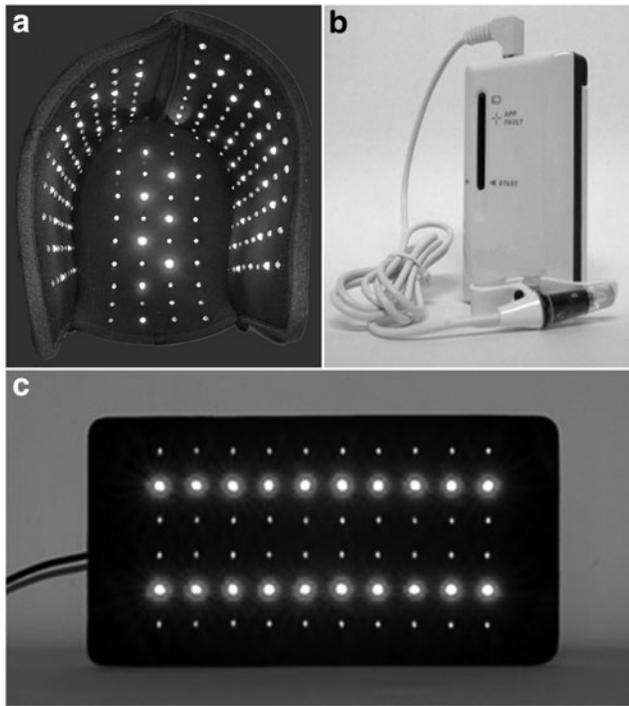
**FIG. 1.** Three types of noninvasive LED devices using red and infrared diodes were used for multi-modality PBM therapy on the patient. (a) Transcranial helmet (ProNeuroLIGHT LLC), (b) intranasal (VieLight, Inc.), and (c) body pad (ProNeuroLIGHT LLC) devices. LED, light-emitting diode; PBM, photobiomodulation.
